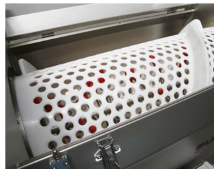
Cilindro forato in polietilene. Polyethylene holed cage.
